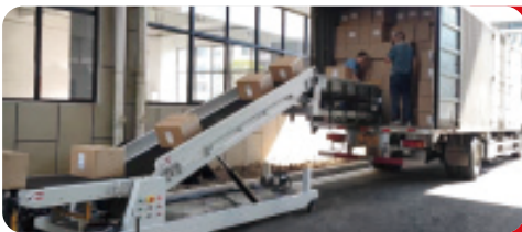
Carton Loading Conveyor
