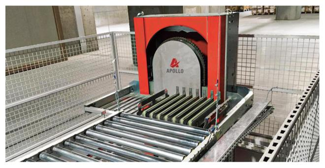
APOLLO can provide customers better logistics solutions with international experience in plant logistics innovation and optimization. Rotative vertical lifter is used for vertical transport and sorting for goods between different floors.
